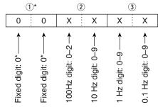
\*Not necessary when setting a frequency.
